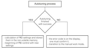
The autotuning process will be broken without PID settings calculations,
