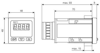
Fig. 2. Controller overall dimensions
