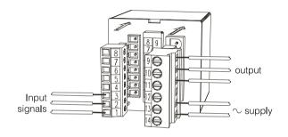
Fig. 3. View of controller connection strips.
