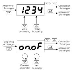
Fig. 9. Setting change of number and text parameters
